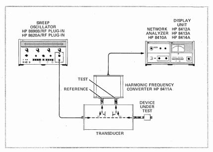
Figure 2-2. Reflection Measurement
