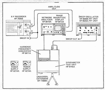
Figure 4-13. Test Setup for Measuring Amplifier Gain
