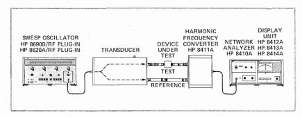
In these basic test setups, the RF signal source shown is the HP 8690B/8620A Sweep Oscillator with the 8690/8630 series RF plug-ins. While all HP sweep oscillators are designed to provide optimal results with the network analyzer system, however, other sweep oscillators are usable if they meet the following specification:
