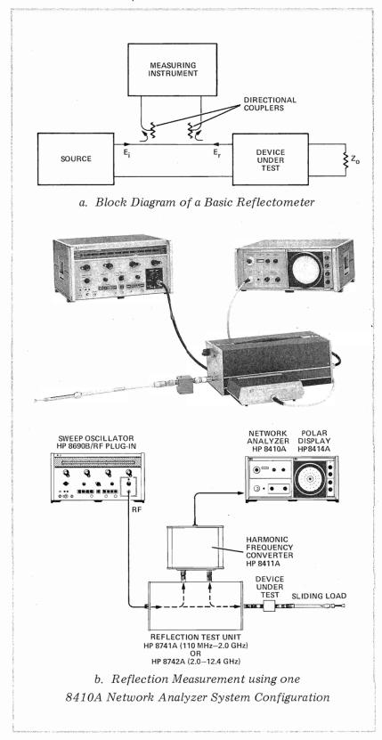
Figure 1-1. Reflection Measurement Test Setup
