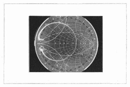
Figure 8-3. Resonant Response of Yig Sphere
