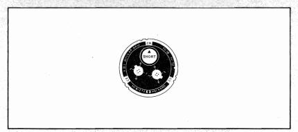
2. Rotate dial so HP is at bottom. Plug in short termination so that the arrow points up, as shown.
