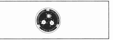
a. Rotate the dial to common emitter (CE). Plug in the transistor making sure the tab on its case fits into the notch on the dial. With the transistor snap-on dial in the common emitter mode, the colored notch on the perimeter of the dial lines up with the "set A" port line on the transistor fixture.
