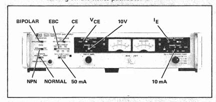
Figure 6-4. HP 8717A Transistor Bias Supply Setup
