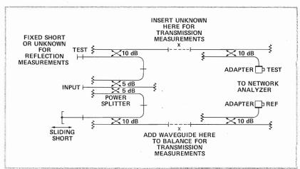
Figure 7-2. HP 8747A Schematic
