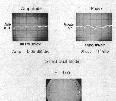
These adjustments are made to calibrate the displays for a through circuit. The Polar Display must show a transmission coefficient  $= 1/0^{\circ}$  and the Phase-Magnitude Display an insertion loss of 0 dB and  $0^{\circ}$ . The Network Analyzer system is now properly set up and calibrated for accurate use.
