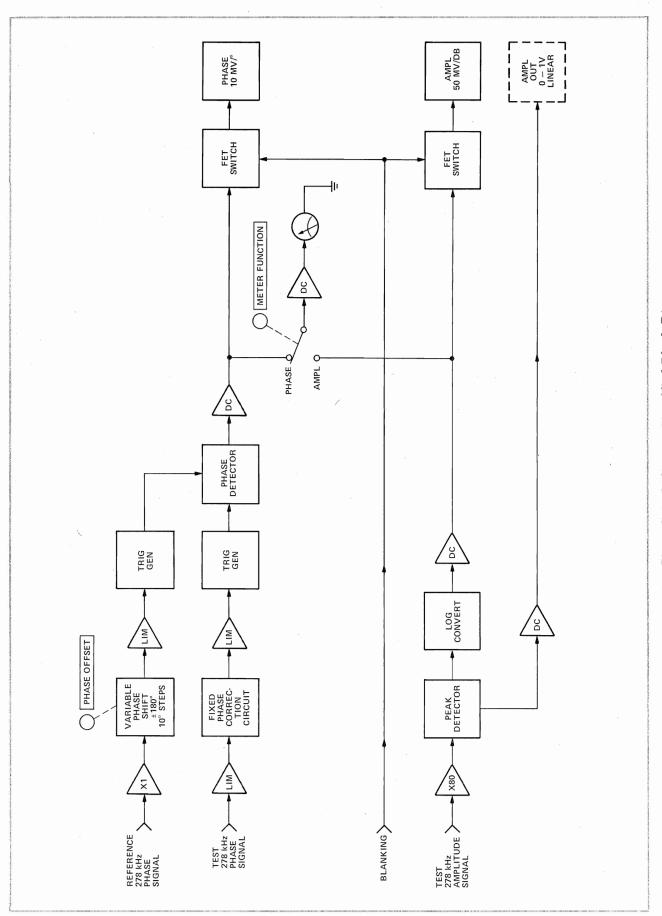
Model 8413A Phase-Gain Indicator, Simplfied Block Diagram
