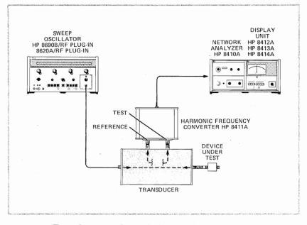
Transducer used in a Reflection Measurement
