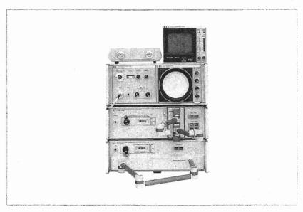
$\begin{array}{c} \textit{Figure 2-16. HP 8410S Option 310} \\ \textit{0.11} - \textit{12.4 GHz} \end{array}$
