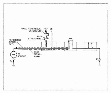
Figure 4-4. Reference and Test Channel Path Lengths
