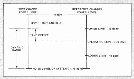
Figure 3-5. Power Levels for Attenuation Measurements
