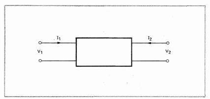
Figure 1-7. Simple Two Port Network
