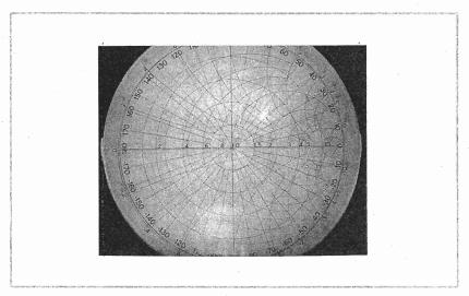
Figure 2-10. Polar Display for Measuring Complex Reflection Coefficients or Impedance with Smith Chart Overlay
