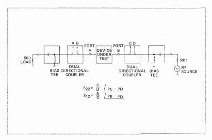
Figure 4-3. Setup for Measuring  $S_{22}$  and  $S_{12}$
