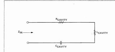
a. Equivalent Circuit of Cavity Alone, Used to Determine Q
