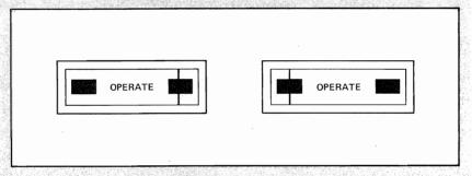
during this test, reduce power from the sweeper. If the needle moves into the left black portion, this could indicate that the system is dropping out of phase lock. Increase RF power or readjust sweep stability control.
