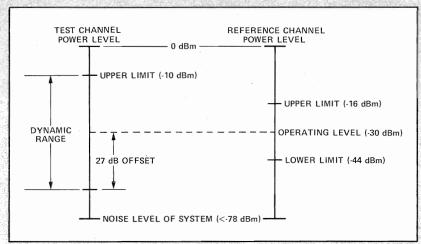
Figure 3-6. Power Levels for Gain Measurements
