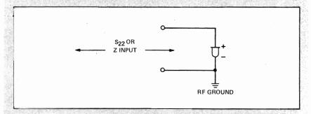
3. Decrease the RF power until there is just enough to operate the network analyzer as indicated by the reference channel level indicator and depress  $S_{2\,2}$  pushbutton.
