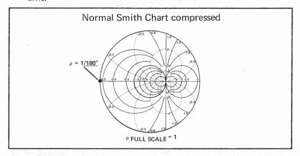
Since a tunnel diode with negative resistance has a reflection coefficient greater than one, reduce the 8410A test channel gain by 10 dB. This makes the outer circle equal to a reflection coefficient of 3.16.
