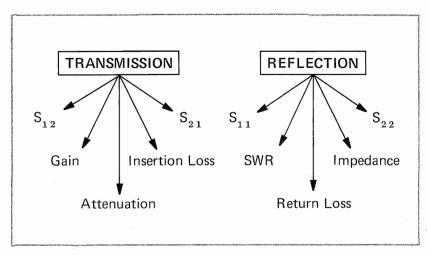
Figure 1-9. Network Parameters from Transmission & Reflection Measurements
