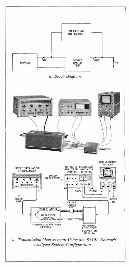
$Figure\ 1\text{--}4.\ Transmission\ Measurement\ Test\ Setup$
