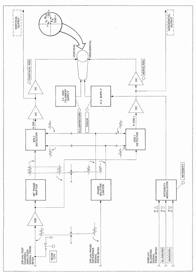
Model 8414A Polar Display, Overall Block Diagram
