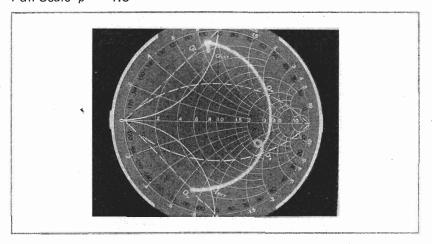
Figure 8-5. Determination of Q of Yig Spheres
