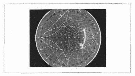
Figure 8-4. Determination of Q of YIG Spheres
