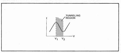
By using markers on the sweep oscillator, the frequency at which tunneling ceases can be determined. To do this, bias the diode for tunneling again and then raise the RF frequency to sweep between 250-500 MHz. By using a marker on the 8690B, the frequency at which  $S_{2,2}=1$  can be determined.
