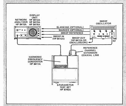
Figure 1. Cable Connections When Using the 8745A
