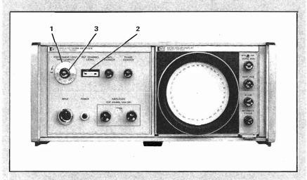
Set sweep of source for an octave band within the frequency range of interest, e.g., 1-2 GHz, and sweep speed to 0.01 sec.
