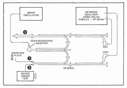
Figure 7-3. 8747A Reflection Test Setup
