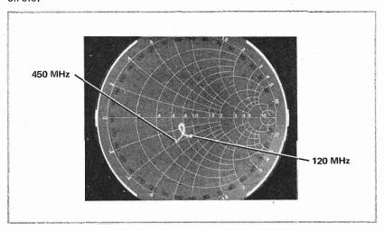
Figure 2-9. Test Result Using the 8414A in a Reflection Measurement.
