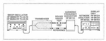
Transducer used in a Transmission Measurement
