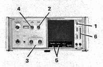
a. Select Phase mode (No. 1) at 90°/div. Adjust horizontal controls (No. 5) for sweep linearity.
