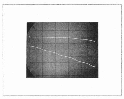
Figure 8-10. Amplifier Gain and Phase
