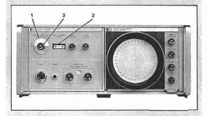
Set sweep of source for an octave band within the frequency range of interest, e.g., 1-2 MHz, and sweep speed to 0.01 sec.
