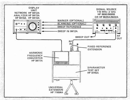
Figure 4-5. General Test Setup for Microwave Hardware Measurements Using the 8745A S-Parameter Test Set \*Rear-Panel Coaxial Link (HP Part No. 11604-20021)
