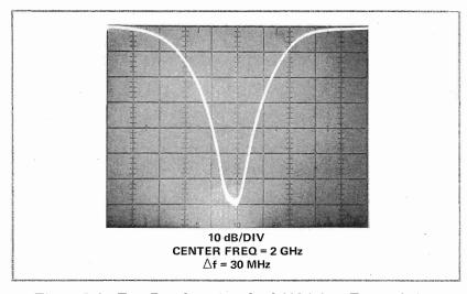
Figure 2-6. Test Results using the 8412A in a Transmission Measurement of an HP 8739A Notch Filter
