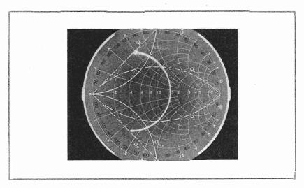
Figure 8-7. Cavity Resonsant Response
