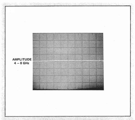
Figure 3-3. Proper Phase Lock
