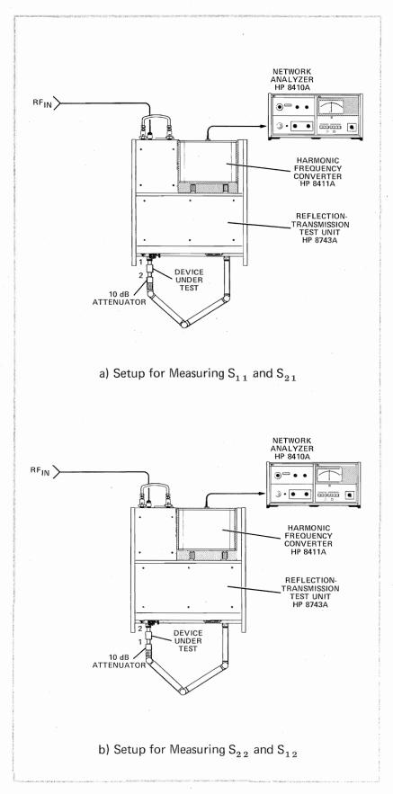
Figure 5-2. Setups for Characterizing Microwave Devices Using the 8743A Test Unit
