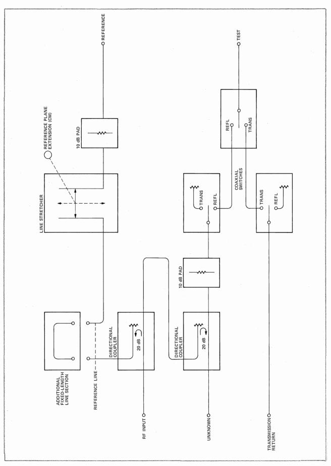
Model 8743A Simplified RF Schematic Diagram
