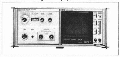
Figure 2-5. The Phase-Magnitude Display Plug-In
