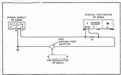
Figure 4-8. Test Setup for Biasing The Pin Modulator
