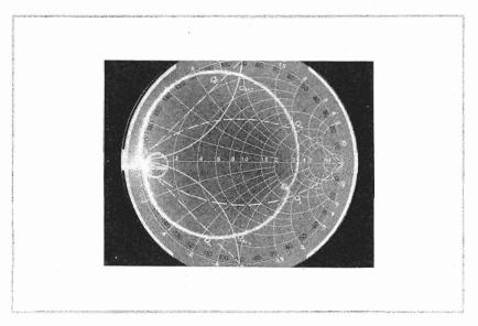
Figure 8-2. Yig Resonant Impedance
