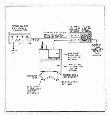
Figure 5-3. General Measurement Setup
