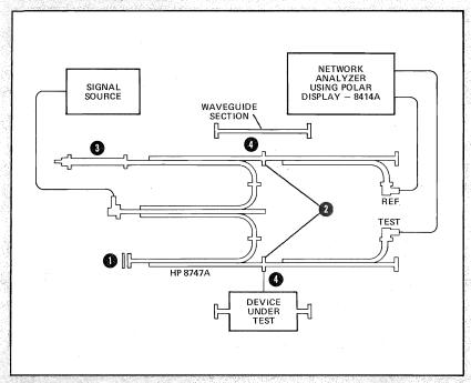
Figure 7-4. HP 8747A Transmission Test Setup
