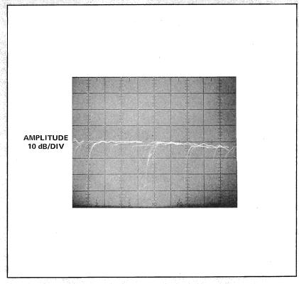
Figure 3-2. Improper Phase Lock
