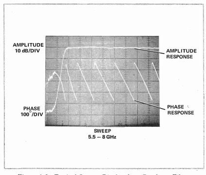
Figure 1-6. Typical Output Display for a Bandpass Filter
